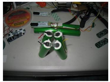
This is the pack, folded in half in the middle. I cut the tabs in such a way to leave each battery enough tab to fold back over itself. This is important, because you cannot solder directly to a cell end, but you can solder to the tab attached to it.
