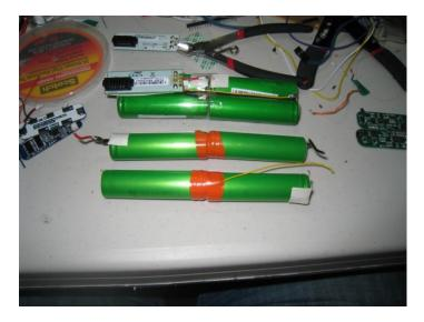
Then tape both rows together in such a way where you can solder one end together, to complete the connection of 4 cells in series. You will need to also add a piece of wire to that junction for later connecting to the protection board. On the other end, solder some heavier gauge wire to the positive and negative terminal, for later connection to the protection board. You can tell which end is positive, as it will have an indented ring around it.
