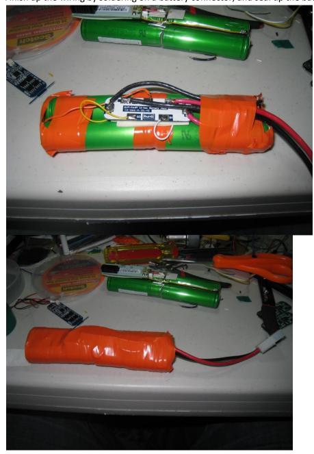
Finish up the wiring by soldering on a battery connector, and seal up the battery in some electrical tape.
