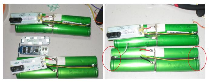
Here we see a before and after. Use side snips to cut the wires at the board, as you are going to want all the length on them later. You can also see the new protection boards on the left. BE CAREFULL TO NOT LET ANY BATTERY ENDS / WIRES TOUCH EACH OTHER!!!
